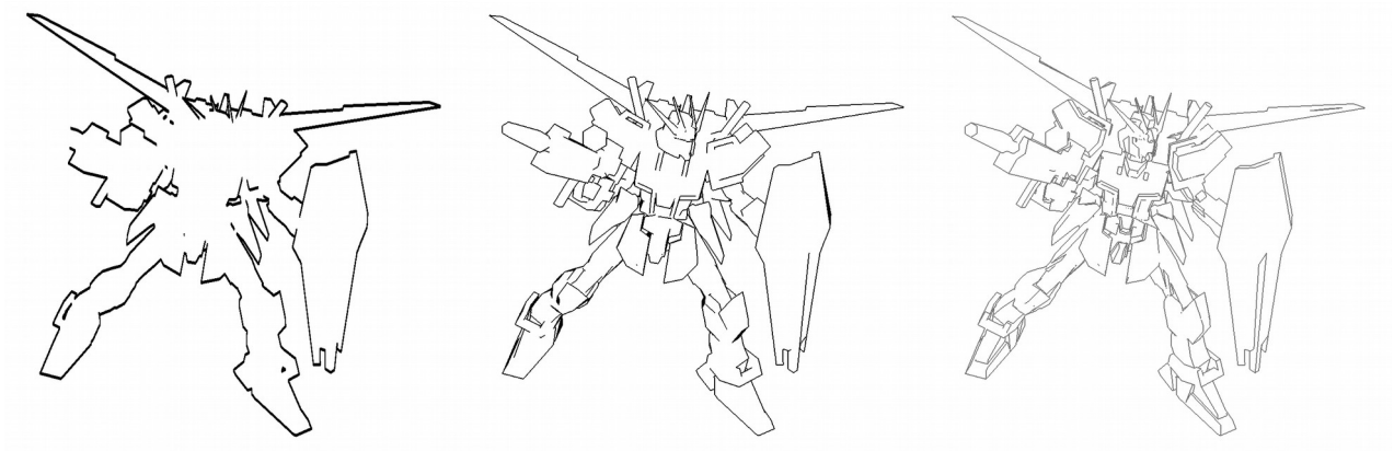
From left to right : Z Buffer (Silhouette) ; Z Buffer (Fine) ; Normal Buffer
